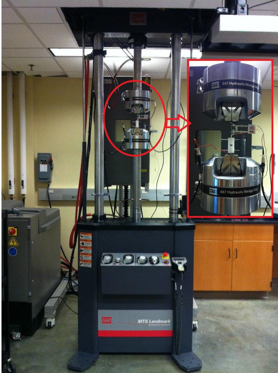
Figure 3.6 MTS Landmark™ and dielectric measurement set-up
