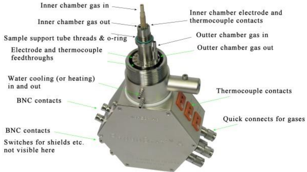
Figure 3.5 Probostat™ base unit with feedthroughs
